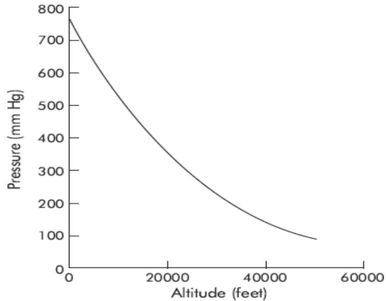
Figure 1 Relationship between atmospheric pressure (mm Hg) and altitude (feet).
